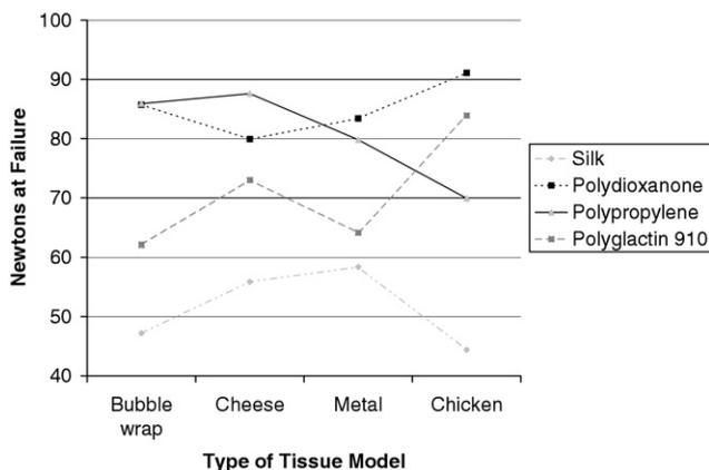
**FIGURE 2.** Mean tension at failure for knot material and jig type.
